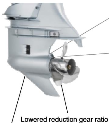
A large diameter propeller of 16" can be installed
